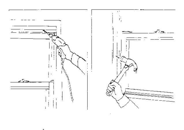
Adjust top expander all the way up if necessary. Caulk around the entire perimeter of the window on the outside, then inside. Replace the old trim strips or install new trim at the head and jambs
