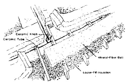
Insulating Around Knob-and-Tube Wiring
